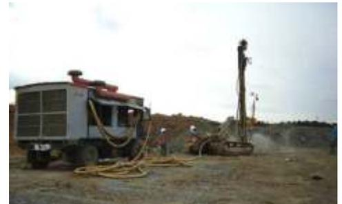
Coal ore mining is preceded by blasthole drilling for opening and loosening of the rock mass. Rock is drilled to open blastholes, where the explosive charges will be placed for blasting. Blasthole drilling is carried out primarily by down-the-hole (DTH) hammer method.
