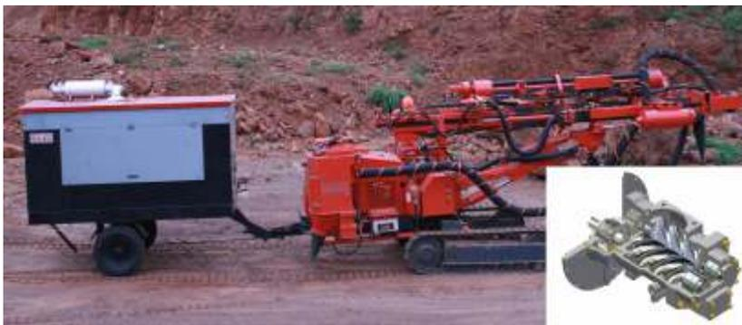
The 159 HP airend has been developed as a reliable solution for the growing high pressure compressed air requirements of segments like mining, construction and exploration. These portable applications necessitate pressures up to the range of 250 psi(g), which is traditionally catered by two stage airends, as single stage airends are limited to a maximum of 200 psi(g) discharge pressure. Overcoming this conventionality, Elgi has developed 159 HP
