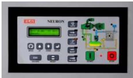
In keeping pace with industry's focus on high-tech advancements, Elgi has developed the Neuron controller with in-house engineering to control medium to large size rotary compressors. This dedicated microprocessor accurately monitors the compressor and ensures precise capacity regulation. The custom designed Neuron controller from Elgi also allows communication capability.
